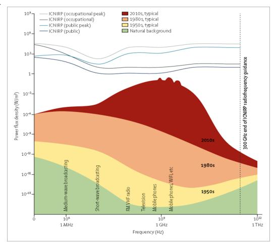
Typical maximum daily exposure to radiofrequency electromagnetic radiation from man-made and natural power flux densities in comparison with International Commission on Non-Ionizing Radiation Protection safety guidelines<sup>1</sup>
